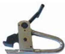
INV2200113 Rim clamp for tubeless truck rims
